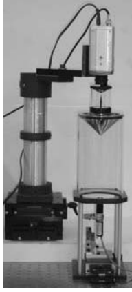
Fig. 1. Structured light-based catadioptric stereo sensor
