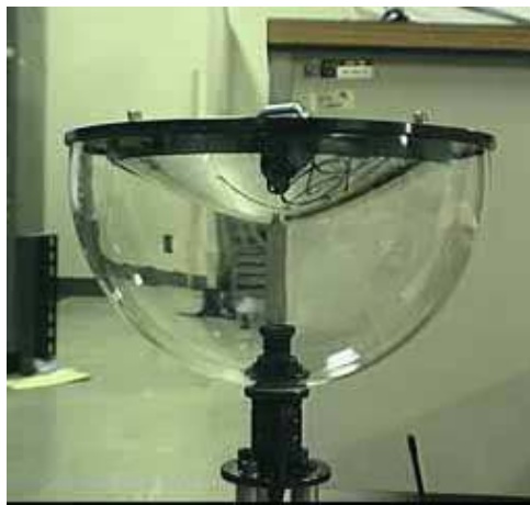
Figure 1.6: Omnidirectional sensor using a hyperboloidal mirror in front of a perspective camera. Courtesy of Yagi, University of Osaka, Japan
