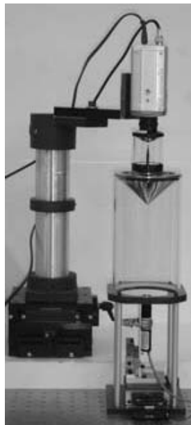
Figure 1.13: Structured light-based catadioptric stereo sensor proposed in [Orghidan et al, 2006]
