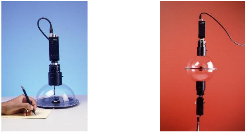
Figure 1.7: Omnidirectional sensor using paraboloidal mirror proposed by Nayar in 1997 with a hemispherical view (left) and entire sphere of view (right)
