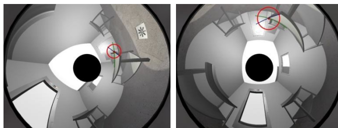
Fig. 5. A synthetic rigid scene. There is a pure rotation around the mirror focal point between two images. The scenes behind the all 4 patches remain the same.
