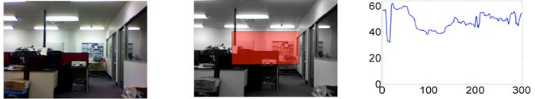
Figure 3.5. Acquired image (left), greyscale image and selected sub-window (middle), and the corresponding image array (right), by [4].
