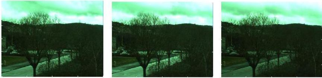
Figure 4.1: Images of a scene recorded with polarizers oriented along 0, 45 and 90 degrees with respect to the horizontal respectively.
