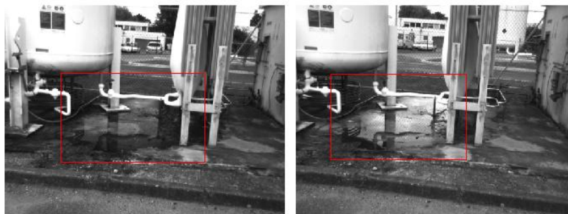
Figure 3.12: Stereo images of an outdoor scene taken from two cameras mounted with polarizers oriented along horizontal and vertical directions highlighting the marked change in intensity of the pixels across the views.
