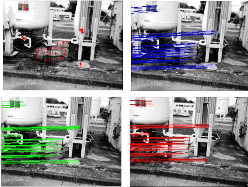
Figure 4.16: The epipolar lines corresponding to the chosen pixels in the top left image are displayed in the other three images.
